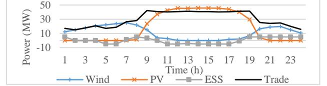
Fig. 3. Power production/consumption of VPP's units and traded power at each period (Case 1).
