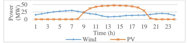
Fig. 2. Wind farm and PV plant power forecast.
