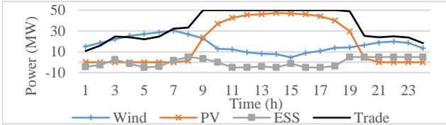
Fig. 7. Power production/consumption and traded power of VPP's units at each period (Case 2).
